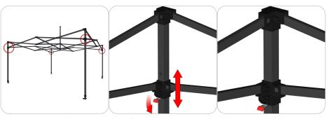
The frame will have four slide locks, one for each corner. When the tent scissor frame is fully extended; make sure the prong of the slide lock snaps into the tube locater hole. Press the lever on the slide lock to disengage the prong from the tube allowing to slide the lock up or down during assembly.
